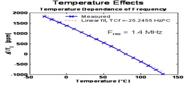
As temperature increases, Silicon becomes less stiff causing the resonant frequency to decrease
